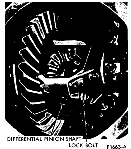
FIG. 5 Differential Pinion Shaft and Lock Bolt
