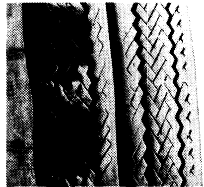
CUPPING—UNDERINFLATION AND/OR MECHANICAL IRREGULARITIES
